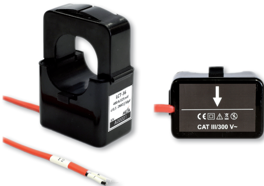
LCT-36 split-core transformer, hole diameter 36 mm
